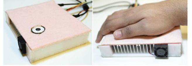
Figure 7. Display with thermoelectric module mounted on a heat sink and fan (left) and with the thenar eminence over the thermoelectric module during stimulus presentation (right).
